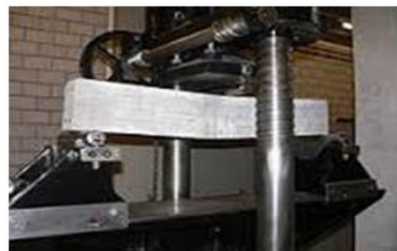
Fig 5.2 Flexural Testing Machine with Prism mould
