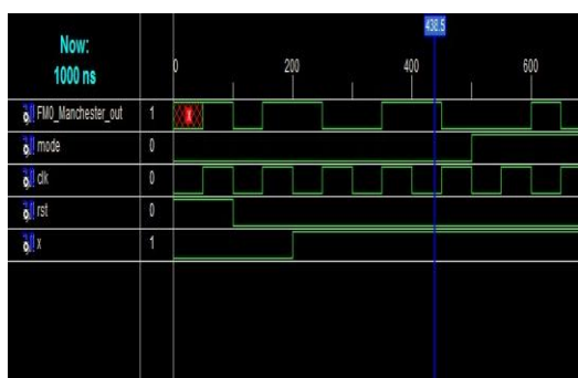
Figure 17: FM0/Manchester encoding using SOLS unbalance technique
