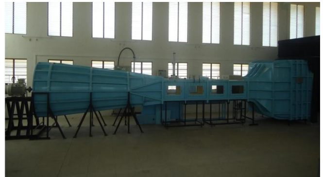
Fig 2.4.1 schematic diagram of subsonic wind tunnel
