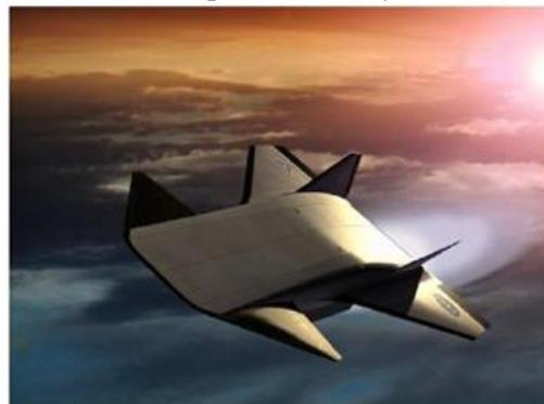
Fig. 3.1 Conceptual design for the X43-A, a reusable hypersonic aerospace vehicle that would utilize UHTC leading edges and control surfaces
