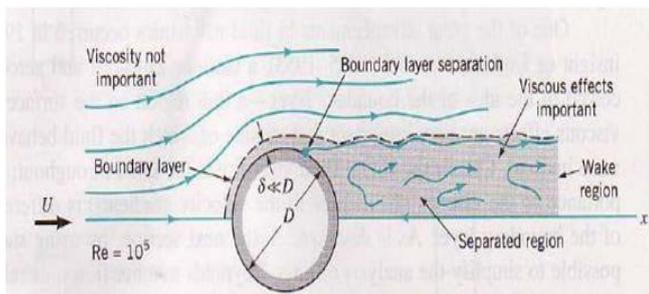
**Figure 1.1: Flow around bluff bodies with flow separation**
