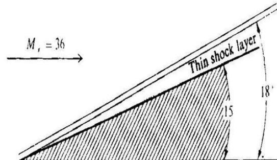
Figure 1.6: Thin Shock Layers
