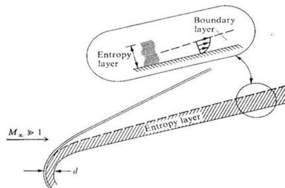
Figure 1.7: Entropy layer near the blunt nose
