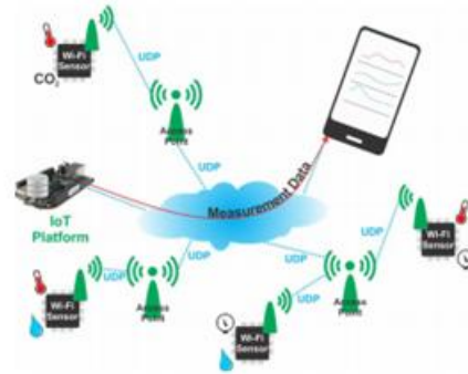
Fig. 1. CPS for environmental monitoring.
