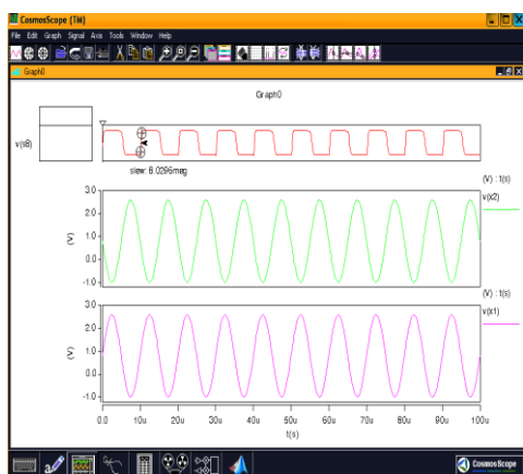
Fig6 (a). Output waveform of Class AB two stage op-amps with current replicating branch using adaptive load I at the input stage.
