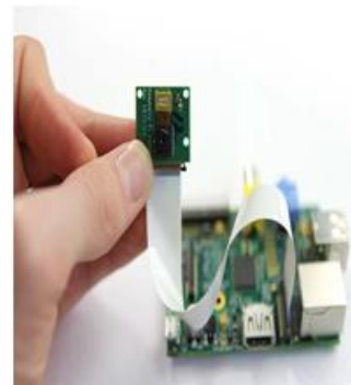
Fig 4: Camera Module Interface to the Raspberry PI
