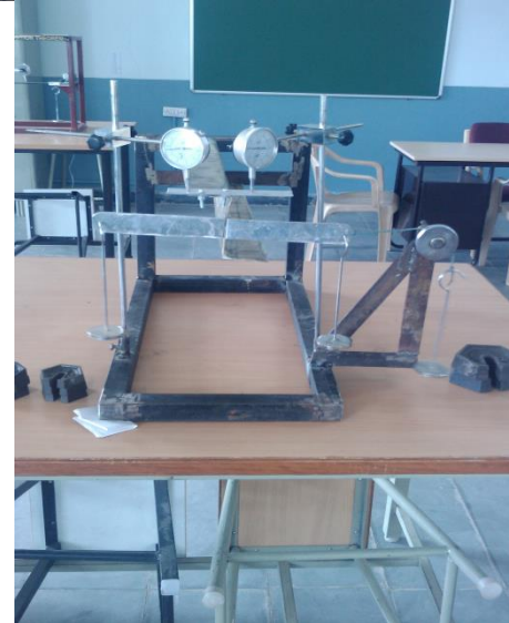
Figure 11: shear centre calculations on Z-section
