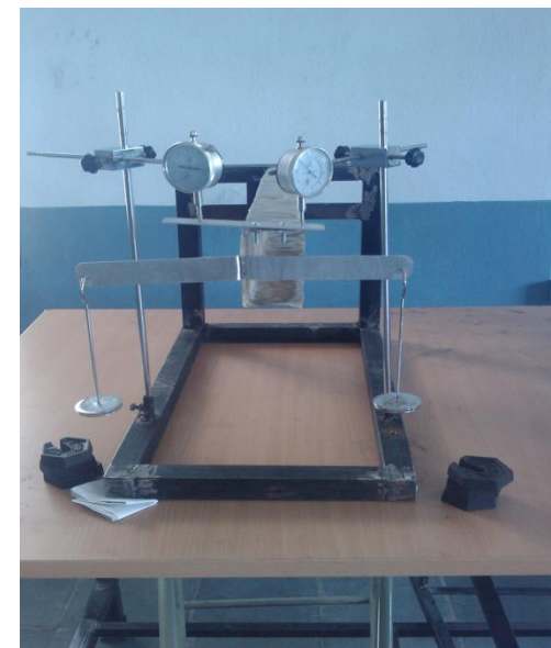
Figure 10: shear center calculations on channel section
