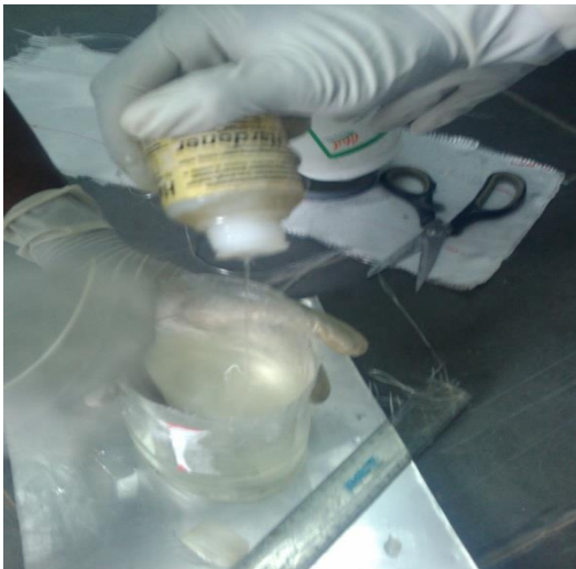
Figure 9: Preparing of composite material
