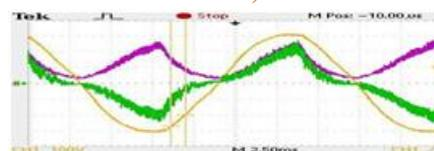
**Fig. 21. Input voltage and current operating with V<sub>i</sub>=220 V<sub>rms</sub> and without the third harmonic reduction technique (CH1 - Input voltage - 100**
