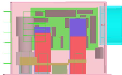
Fig 3.4: components ICEPAK Geometry
