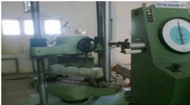
Flexural Strength Test
