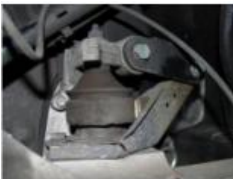
Fig: engine mounted on engine mount
