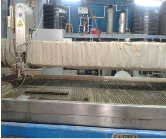
Fig – Setting of work piece on the machine
